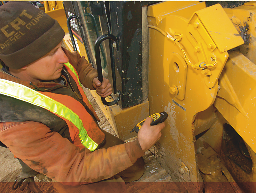
A Ryan Inc. field mechanic swipes a machine's bar code with a cell phone and reader accessory before filling the fuel tank. Fuel pumped, together with machine hours keyed into the phone's keypad, allows Ryan to monitor and manage fuel consumption for each machine in its fleet.
