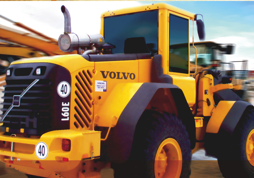
Volvo dealers are selling the HUSS M-K diesel particulate filter as a Volvo-approved product. The active-regenerating filter has a diesel burner that clears accumulated soot from the media. The M-K is a Level-3 VDECS for on-road and off-road engines from 50 to 750 horsepower, in rubber-tired and tracked applications.
